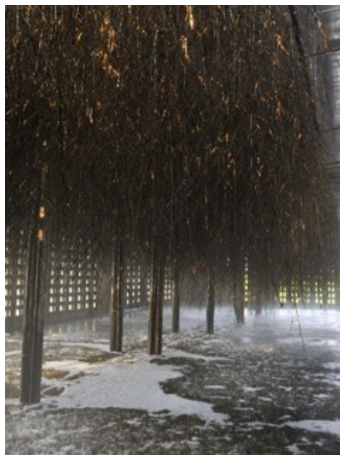
Seawater is condensed into kansui inside
