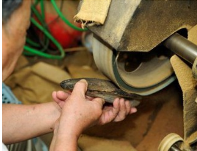
Hadakabushi is made by trimming off the charred surface of arabushi
