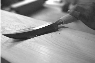
The curved, razor-sharp yari-ganna, or spear plane, is but one of the traditional tools that the miya-daiku must master. (Courtesy Mitsunari Sakurai)
