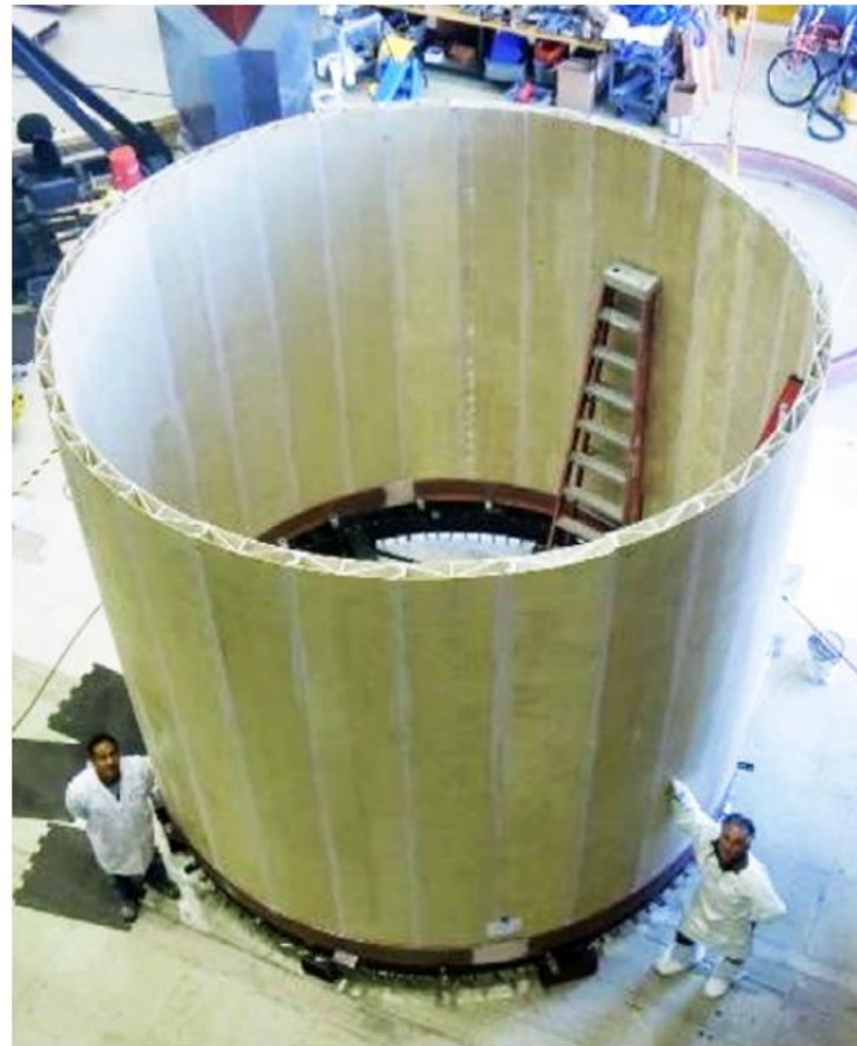
Figure 8.2 Lockheed Martin's CWP R&D programme with a 4 m pipe next to two engineers
